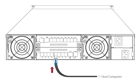
8. The US\_PM-2425 enclosure is with redundant PSU, so connect one end of the two power cords to the two power receptacles at rear of US\_PM-2425 enclosure, and then connect the other end of the two power cords to the power outlets.
