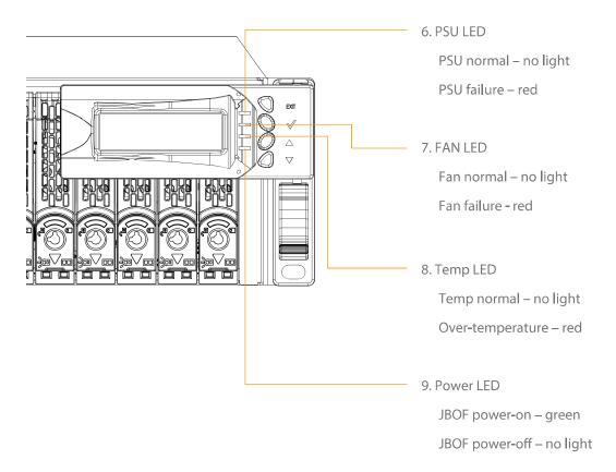
Use the Down/Up button to move downward/upward, browse the selection, and select the item. Press Enter button to confirm the selected item; press Return button to go back to the previous display of screen.
