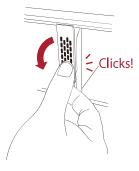
※ Do not force the levers to close while you insert U.2 drive modules into the enclosure. If a lever does not close smoothly, draw out and insert the U.2 drive module again, and then press the lever to close. 6. Repeat steps 2 to 5 for further U.2 NVMe SSD drives.
