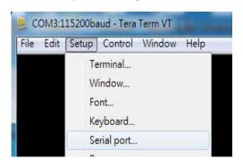
For "Port", select COM3 in this example. (Depends on which COM port used on Host)
