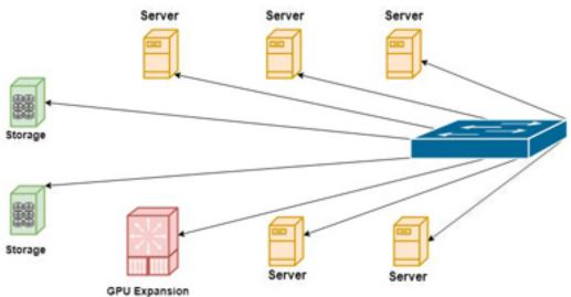
For host to host communication, the PCI-SWG3-024E can be combined with PCI-AD-x16HE-MPS Host Adapters. Operating in Non-Transparent Bridging mode, Serial Cables has solved the strict power on requirements normally associated with PCI Express. Hosts, cables, and the switch can be hot-swapped and power cycled in any order, providing real plug and play as normally expected from networking components.
